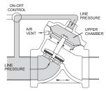
**DRIP-TIGHT CLOSING:** Closure is obtained by directing line pressure or equivalent independent pressure into the upper chamber. This pressure on the large diaphragm area causes the valve disc to seal against the seat.
