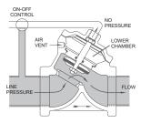
**FULL OPEN OPERATION:** When the closing pressure in the upper chamber is relieved by venting the pilot line, the valve opens positively, by line pressure on the disc.
